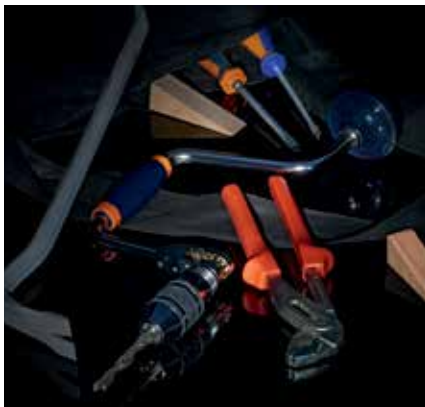
Image on right: Break-in tools according to the RC 3 security class
